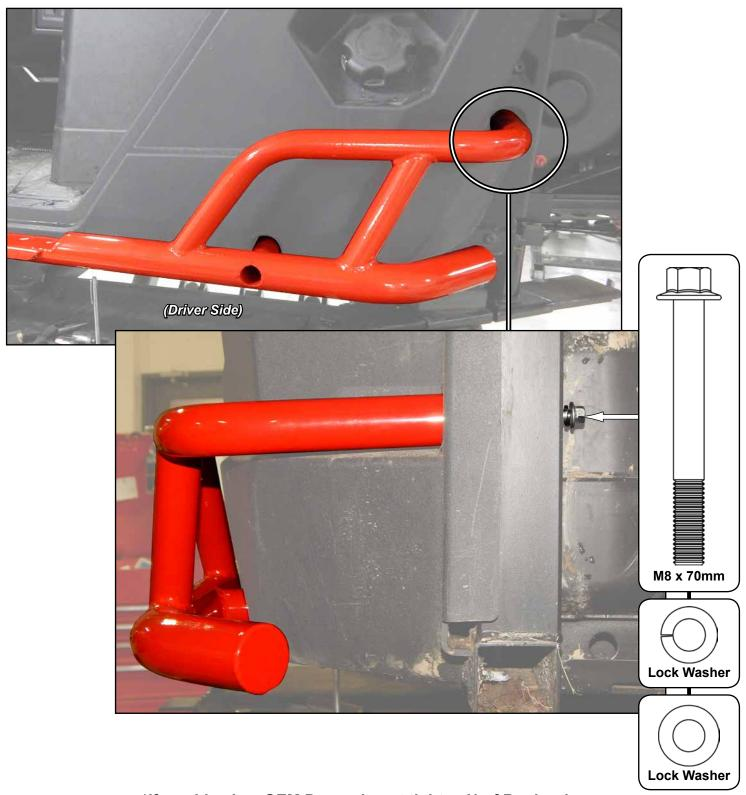
\*If machine has OEM Doors do not tighten Nerf Bar hardware until Doors have been adjusted for clearance.
